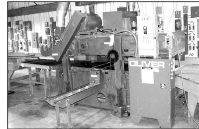
Oliver 170 Double Sided Strait-O-Plane Helical Carbide Cutterheads
