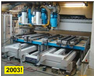
Shoda Titanium Twin Table CNC Router & Vert/Horz. Borer w/ (2) Tool Changers
