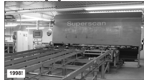
Grecon Super Scan 2D Rip Optimizing System With Chain Decks, Prog. Fence
