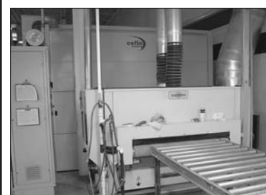
Sorbini Cefla UV Spray Line w/ Panel Cleaning Brush, Denibbler, & UV Curing Ovens
