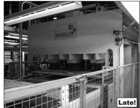
Burkle Heavy Duty Press Line w/ Glue Spreaders
