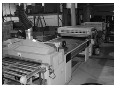
Elmag Superfici Roller Coating Line w/ UV Ovens
