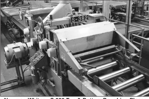
Newman Whitney S-382 Top & Bottom Roughing Planer w/Newman Spiral Quiet Cut Heads
