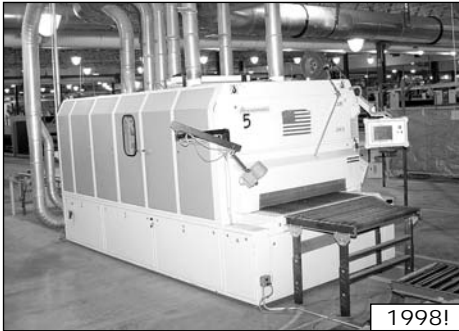
Heeseman LSM-8 Wide Belt Sander w/ Sensing (Platen, Cross Belt, Cross Belt, Platen, Platen, Platen, Panel Cleaner, Installed in 1999)
