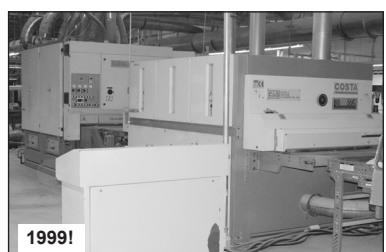
1999! Costa Top & Bottom Sanding Line
