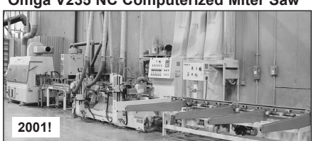
2001! Makor Sanding & UV Finishing Line: Makor Loader/Transfer, Wheel Sander, Transfer Conveyor W/Vacuum UV, UV Oven, SCS Unloader (All 2001) & Dustek Collector (2002)
