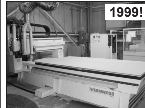
Thermwood C-53 CNC Router w/ Tool Changer, 60" x 12' Table
