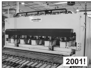
Sennerkov Hyd. Press Laminating Line w/ Programmable Controls
