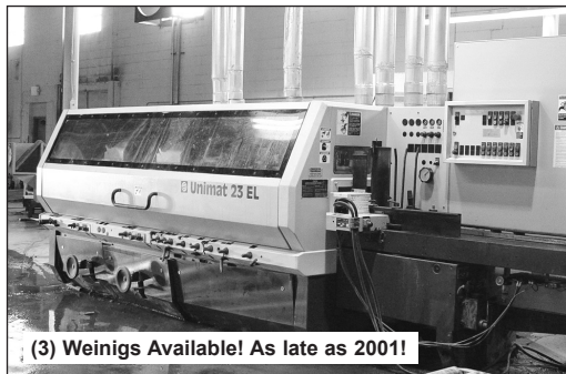
Weinig Unimat 23EL Moulder w/ Tilting Side Head
